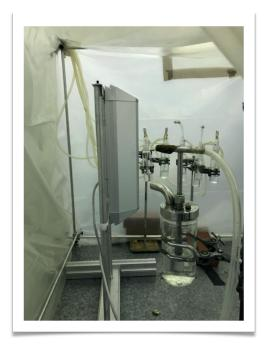
PLACEMENT OF THE DEVICE, NEBULISER AND IMPINGERS IN THE ENCLOSURE
